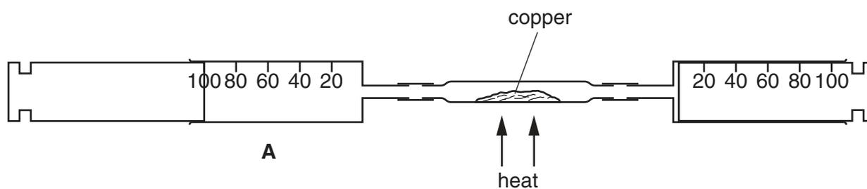
Syringe **A** contains  $100\text{ cm}^3$  of air. The air is forced backwards and forwards over the heated copper until the volume of gas forced back into the syringe **A** is constant.
